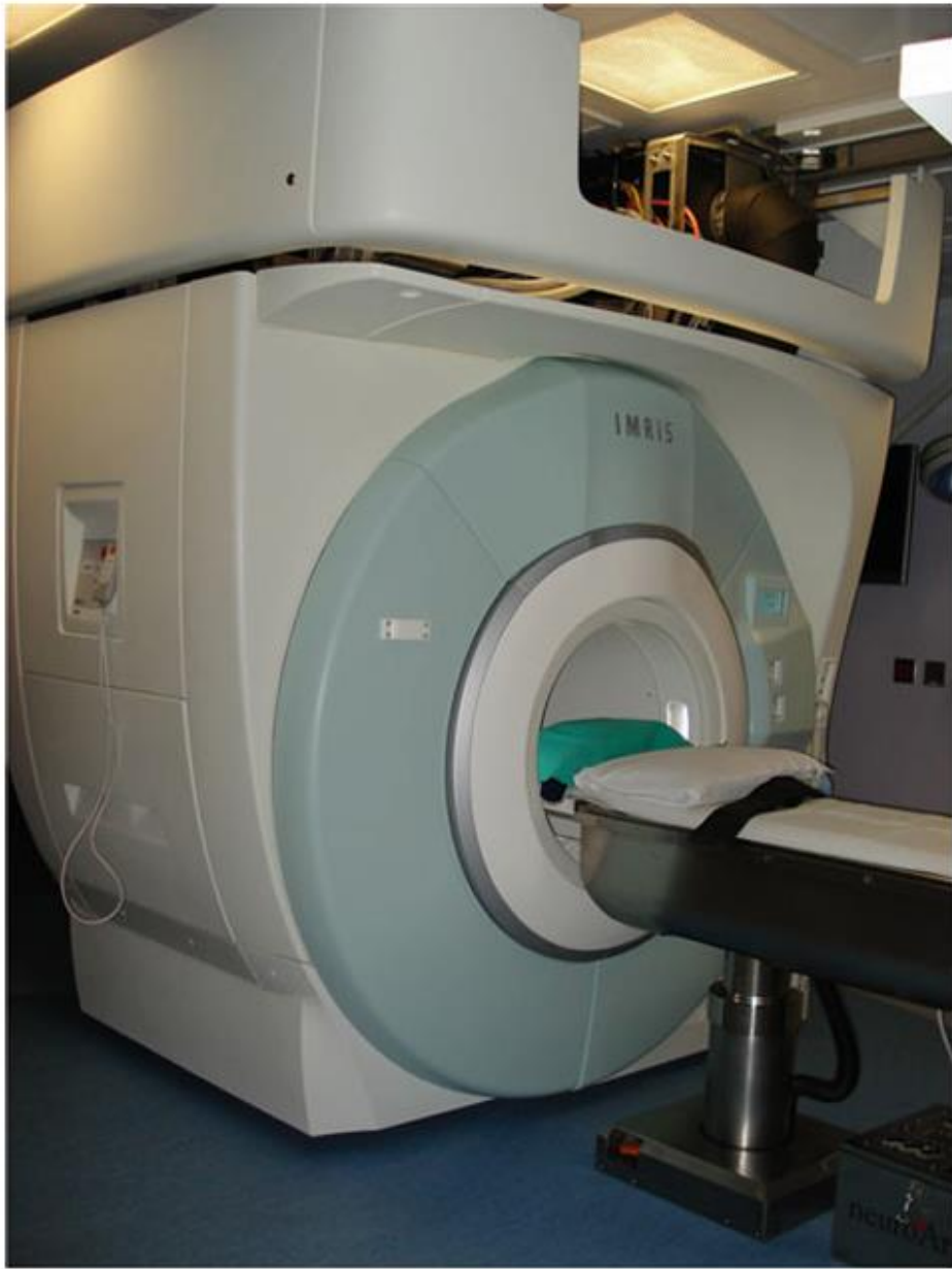
Fig. 3 IMRIS 1.5 T intraoperative magnetic resonance imaging system with the magnet suspended from ceiling rails. In the foreground is the MRI-compatible surgical table
