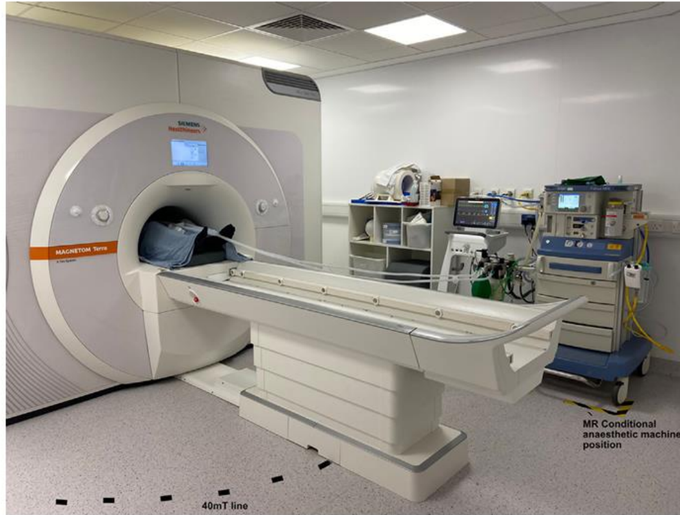
Fig 1. Anaesthetic set-up for ultra-high-field anaesthesia, including an MR conditional Fabius MRI Dräger anaesthesia machine (Dräger, Lübeck, Germany) and Philips Invivo MR400 monitoring system (Philips, Amsterdam, The Netherlands) around a 7T Siemens Magnetom Terra scanner (Siemens AG, Munich, Germany). The black and yellow dashed lines represent where the MR conditional anaesthesia machine should be positioned. The black dashed line around the MRI scanner represents the 40 mT line.
