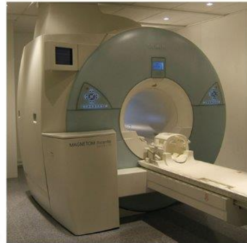
Figure 1. Appearance of the clinical MR scanners used. a: Conventional MR scanner with a flat front and a bore with a length of 2.25 m and a width of 0.6 by 0.53 m. b: Recent MR scanner with a short (1.6 m) and wider conical-shaped magnetic bore (0.6 m).
