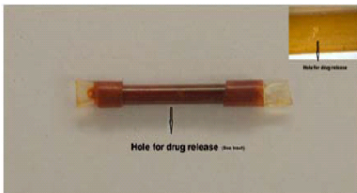
Figure 1. The drug delivery system with microhole on the surface. Hole diameter = 200 \mu m; Tube diameter = 1.8 mm; Tube length = 20 mm. The size of the device and the perforations can be scaled to fit the need of the therapeutic application [12].
